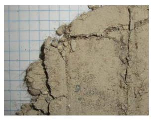
Close up image of interior plaster sample. Note higher clay content with hair reinforcement. (ERA).
